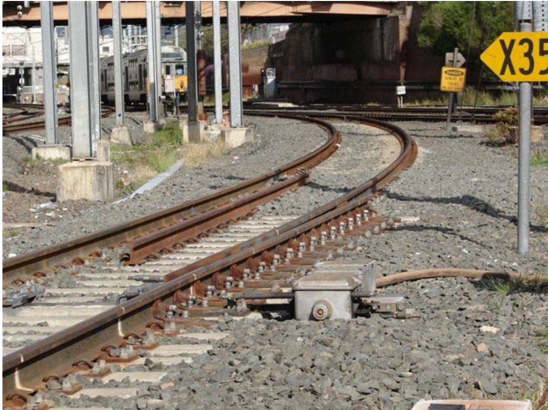
Picture 3: Granville 710 catch point with guard rail arrangement Picture taken with back to country, showing only part of guard rail installed
